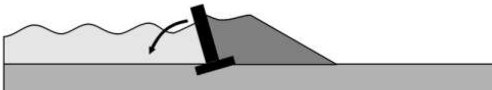
Tilting of walls due to differential settlement
