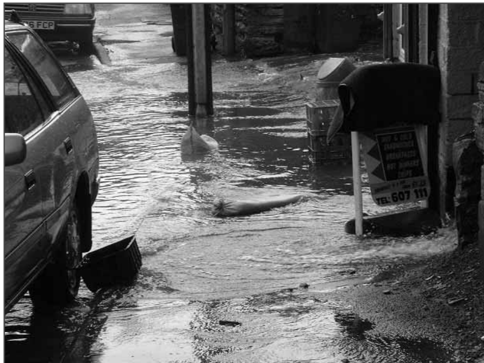
Figure 2.2 Conveyance of exceedance flow in surface flood pathways (courtesy Pennine Water Group)
